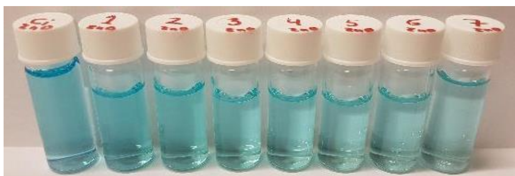
Fig. 5. Degradation of methylene blue with ZnO – sample. The 7th sample (right) was taken after 2h and 15min. This was shown to the students during the microplastics station.
