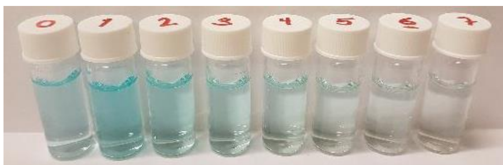
Fig. 4. Degradation of methylene blue with ZnO/SnO/Fe^0 – sample. The 7th sample (right) was taken after 2h and 15min. This was shown to the students during the microplastics station.
