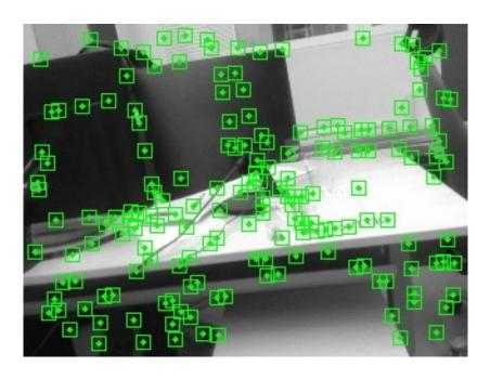
Notice how the GCNv2 features have a more even distribution of features than ORB Can run ORBSLAM2 with GCNv2 on Jetson TX2 https://github.com/jiexiong2016/GCNv2\_SLAM
