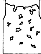
Micro Porosity (Interdendritic porosity)
