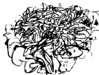
Figure 6.10 (a) Graphite crystal, which grows radially from a centre, forms a cell.
