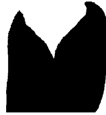
Figure 10.35 'Fish-tail'. From K. Strauss, Applied Science in the Casting of Materials, reproduced with kind permission of Foseco International Limited.
