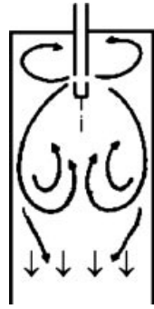
Figure 3.17 Flow pattern of the melt around a casting tube in the mould.
