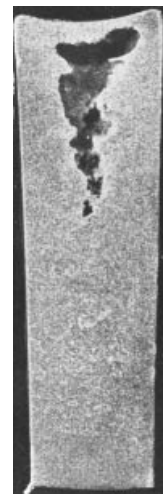
Figure 10.29 The appearance of the pipe in an ingot with equiaxed crystal structure.
