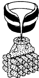
Figure 1.6 (e) Casting is performed directly into the hot mould. Reproduced with permission from TPC Components AB.
