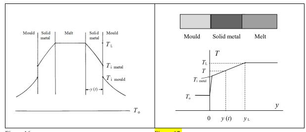
Figure 16. Temperature distribution in mould and metal at poor contact at the interface at the time *t* after the casting.
