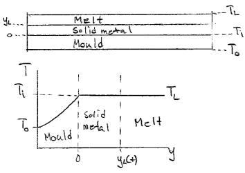
In sand mould there is poor thermal conductivity in the mould rotative to the conductivity in the solidified metal. So  $T_i = T_L$
