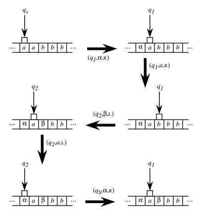
Figure 6.5 The first five steps of the machine of Example 6.4 with input *aabbb*
