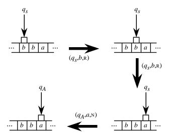
Figure 6.2 An accepting computation path of the machine of Example 6.1
