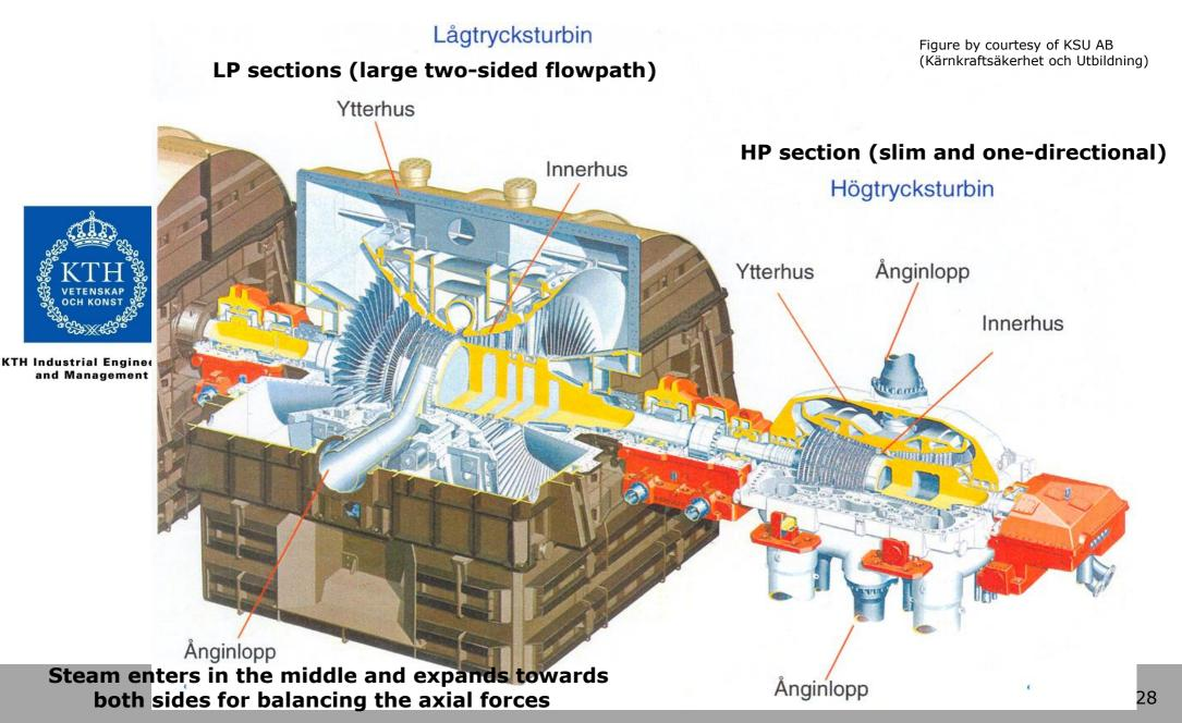
It's critical to keep the long and heavy rotor in perfect balance, without wobbling or bending from thermal or mechanical stress
