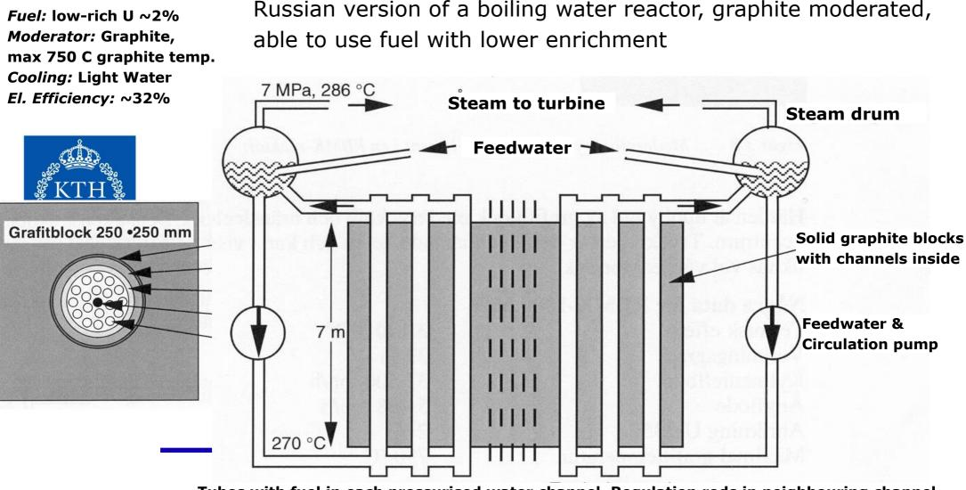
Tubes with fuel in each pressurised water channel. Regulation rods in neighbouring channel. Modular construction. More graphite blocks with tubes can easily be added.
