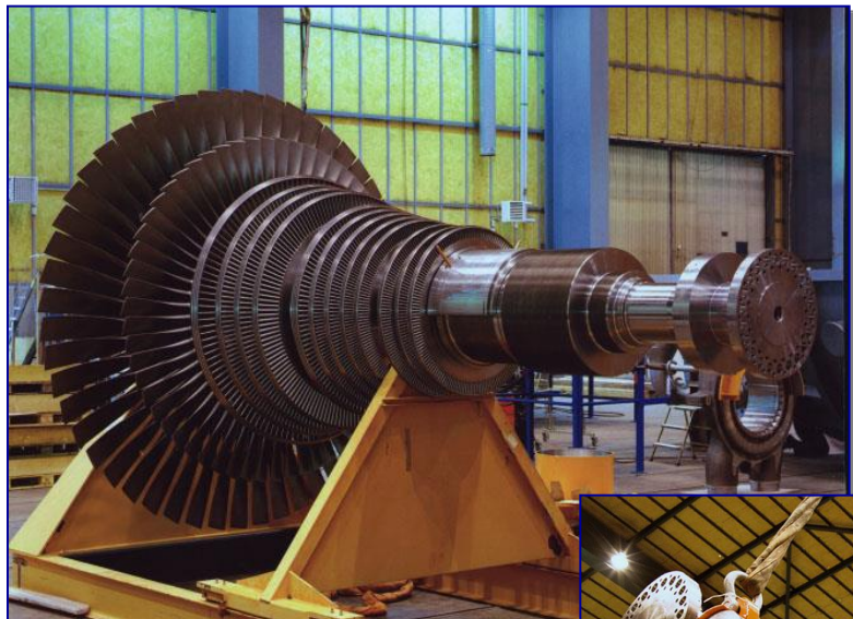
One 114 MW reheat unit in combined cycle. Inlet 148 bara/ 2150 psia, 565°C/1050°F, with reheat to 565°C/1050°F. Order spring 1999.
