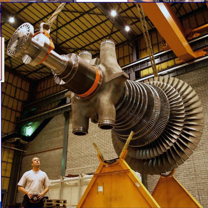
Three 112.7 MW units in combined cycle with W501F gas turbines. Inlet data per unit 112.7 MW at 145 bar(a)/ 2103 psia and 561.3°C/1004 °F. Order 1998.
