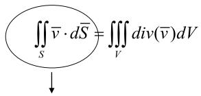
This term is the gas volume per second [m³/s] that flows outwards (or inwards) through a closed surface S
