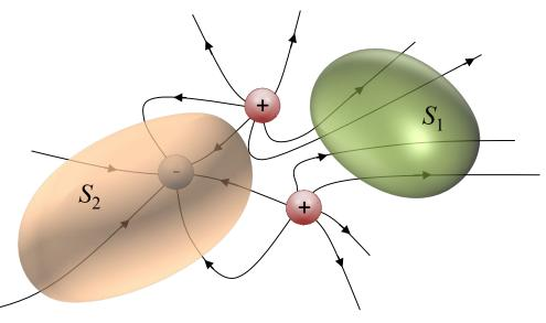
S<sub>1</sub> does not contain any charge. It has no sources and no sinks: no field lines destroyed and no field lines created inside S1
