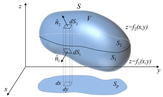
$$\begin{aligned} dxdy &= dS_2 \hat{n}_2 \cdot \hat{e}_z = d\overline{S}_2 \cdot \hat{e}_z \\ dxdy &= -dS_1 \hat{n}_1 \cdot \hat{e}_z = -d\overline{S}_1 \cdot \hat{e}_z \end{aligned}$$
