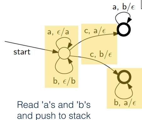
Label "x, y/z" on edge: Read x, pop y from stack, push z
