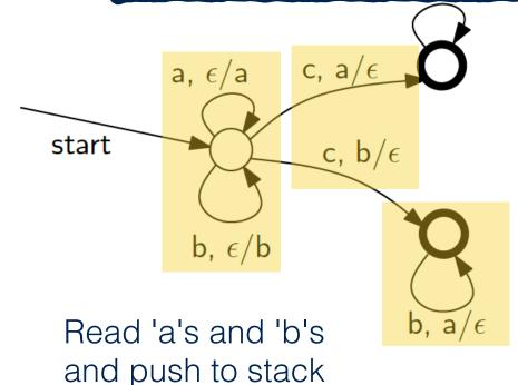
When reading a 'c', jump to one of the accepting states depending on whether the top-most character on the stack is 'a' or 'b'
