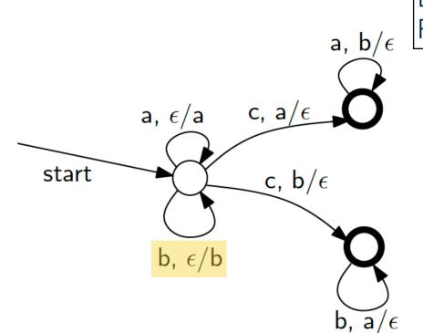
Label "x, y/z" on edge: Read x, pop y from stack, push z
