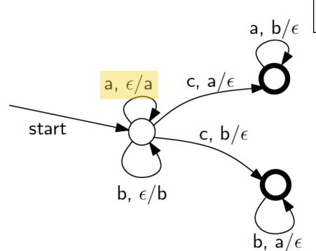
Input: b<mark>a</mark>abcbbb Label "x, y/z" on edge: Read x, pop y from stack, push z
