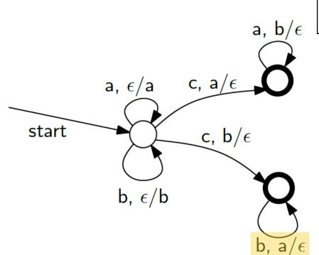
Input: baabc<mark>b</mark>bb Label "x, y/z" on edge: Read x, pop y from stack, push z
