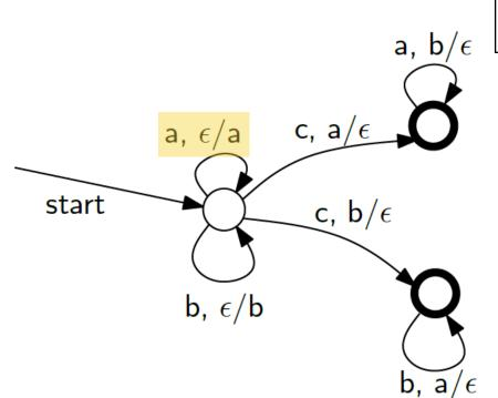
Input: ba<mark>a</mark>bcbbb Label "x, y/z" on edge: Read x, pop y from stack, push z
