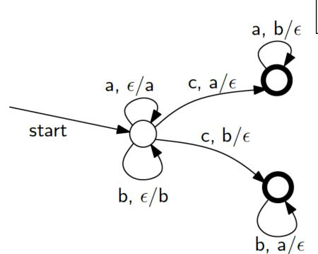
Input: baabcbbb Label "x, y/z" on edge: Read x, pop y from stack, push z
