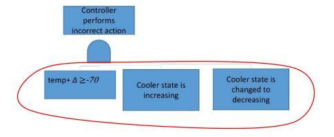
Always after controller reacted if sensor is OK and temp +  $\Delta \ge -70$  then cooler is in decr
