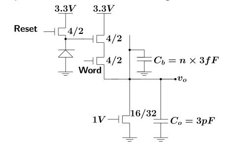
Let's compute the output voltage swing  $v_s$ . The minimum output voltage  $v_{omin} = v_{bias} - v_{TB} = 0.2 \text{V}$ The bias current using  $k_n = 188 \mu \text{A}/\text{V}^2$  is  $i_{bias} = 1.88 \mu \text{A}$ , and the maximum output voltage is
