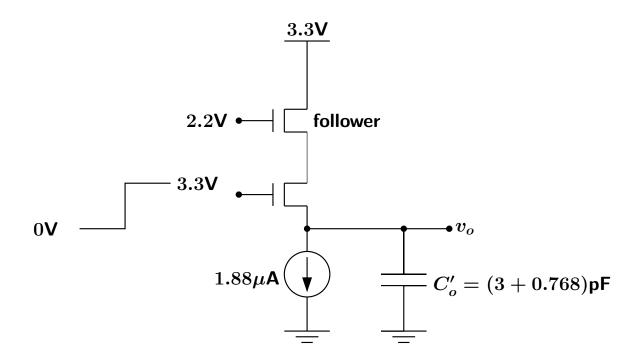
Define the row transfer time  $t_{row}$  as the time from the access transistor turning on to the output voltage  $v_o$  reaching to within half a bit of its steady state value, i.e.,
