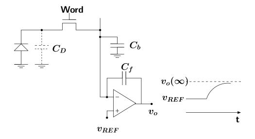
In steady state, assuming charge Q<sub>sig</sub> (electrons) accumulated on the photodiode at the end of integration (and ignoring "feedthrough" voltage added when the reset transistor is turned off and opamp offset voltage), the output voltage
