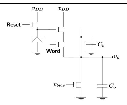
• Assuming charge  $Q_{sig}$  is accumulated on the photodiode at the end of integration, soft reset is used, and ignoring the voltage drop across the access transistor, then in steady state, the output voltage
