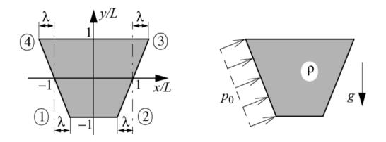
**6.9** Calculate the contribution from the force per unit volume  $K_y$  to the nodal force vector in the above problem by use of numerical integration based on Gauss-Legendre quadrature. Use: (a)  $1 \times 1$  and (b)  $2 \times 2$  point integration scheme in the element.
